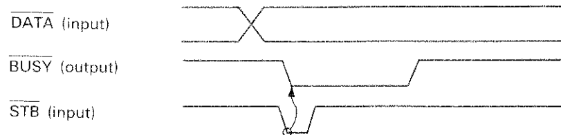
Fig. 5.3.3.A Synchronous Input Timing
